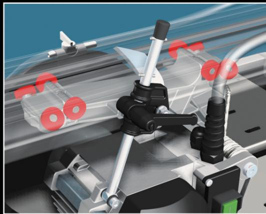
The carriage engine group slides with 8 ball-bearings on interchangeable stainless steel track. So doing the sliding is very fast and precise.
